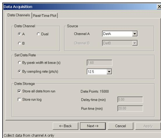
*Data Channels tab for a LINK-controlled instrument*
