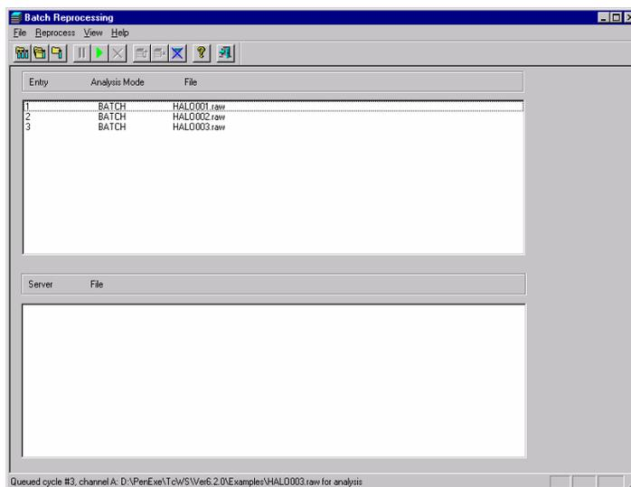
8. Choose Start from the Reprocess menu to begin reprocessing the data. You can also start the Batch process by clicking on the green arrow on the toolbar. The entries on the list are deleted as they are processed. The report and replot for each file will be printed once data analysis is complete.
