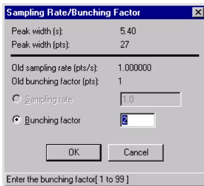
TotalChrom has calculated a recommended bunching factor of 2 in the example above (compared to the old bunching factor of 1 from the default method).
