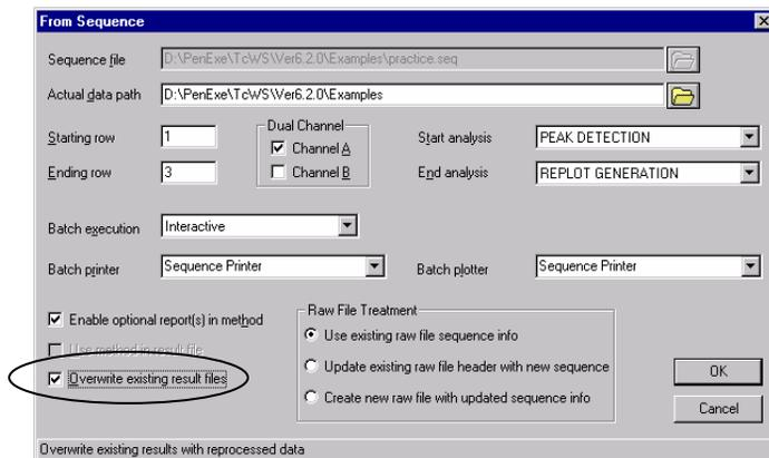
The Batch Reprocessing window opens, listing the raw files that are scheduled for reprocessing. They are the three files from our sequence.
