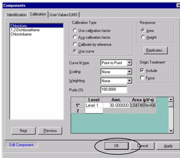
Notice that the area has been calculated and is displayed at the bottom right of the window.
