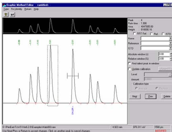
9. For the component name for peak 4, enter 1,2-Dichloroethene.
