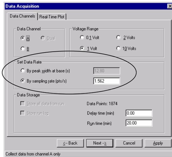
If you know how wide your narrowest peak is at its baseline, select “By peak width at Base” and enter the number of seconds in the text box. TotalChrom will use this to calculate the optimum sampling rate for that peak.
