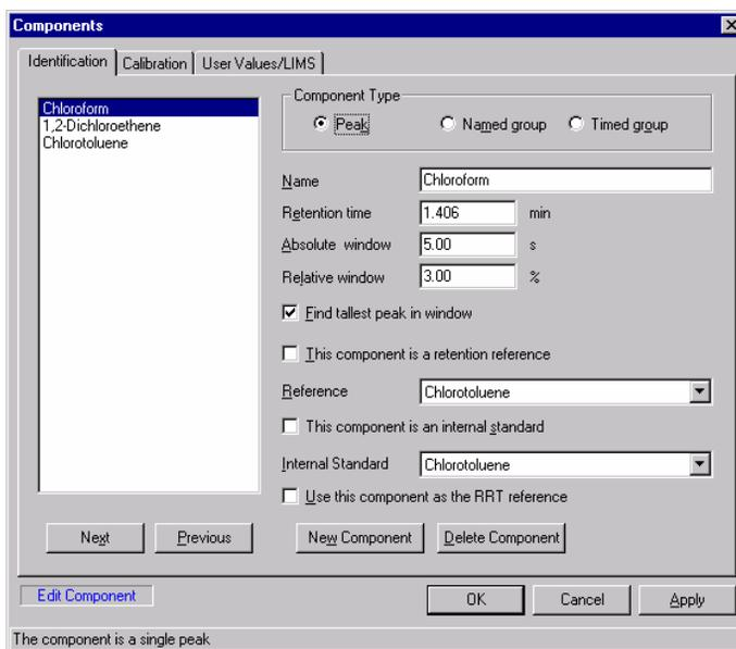
The names of the components that we want to identify in the analysis are on the left side of the window. Information for the selected component is on the right side. We will edit this existing information to add a calibration level for each component.
