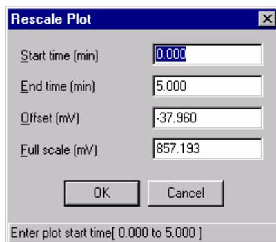
Under Voltage Axis, the value for Full Scale is the value that is currently being used for the display. That value may be (a) from the method, (b) as altered by zooming, or (c) as you specifically changed it in this dialog box.
