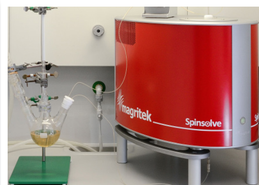
Flow reaction monitoring setup
